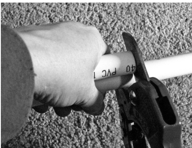
Figure 7 After cutting one pipe by measuring, it's easy to cut matching parts by using the first one as a guide.
