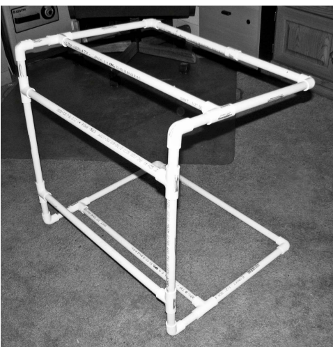
Figure 14 The basic C-shape support assembled. Additional Cs could be added if a wider support is needed.
