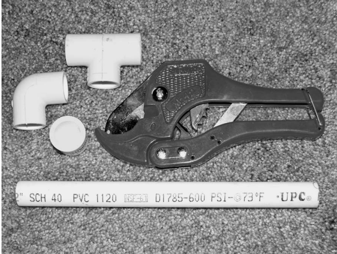
Figure 6 Items to buy include elbow joints, t-joints, end caps, pipe, and a PVC cutter.
